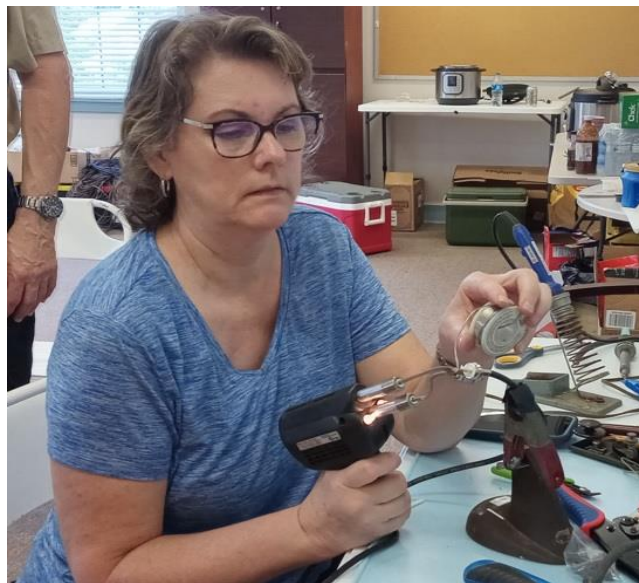
Barbara Mathews soldering the tip on a crimp-on PL259 connector
